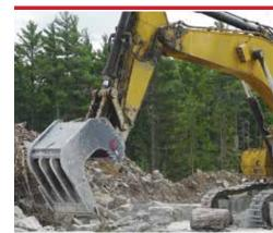
Specialized Limestone Bucket with patented. clamp-in cutting edges. Increased limestone slab production over 100%.
